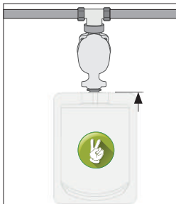
Screw until the edge of the bag is close to the pump inlet
