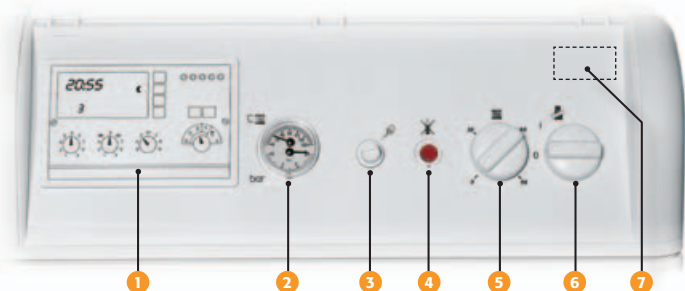
1 Lodging for optional electronic controller 2 Hydrometer 3 Plug (for Pegasus F3) or flues thermostat cover (other models) 4 Flame controller reset button with shutdown light 5 Boiler control thermostat 6 On-Off-Test switch 7 Safety thermostat (with manual reset for 2S models, inside the panel with automatic reset for mod. 56)
