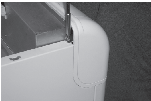
Fig. 8 - Unscrew and take out the two screws and both plates holding the control panel.
