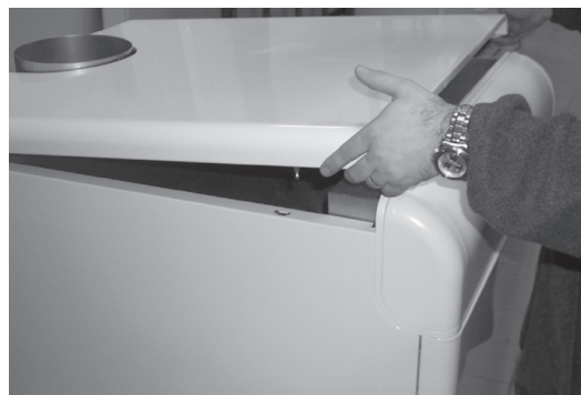
Fig. 7 - Lift by pressing upwards and take off the cover that is held at the sides of the boiler by pins.
