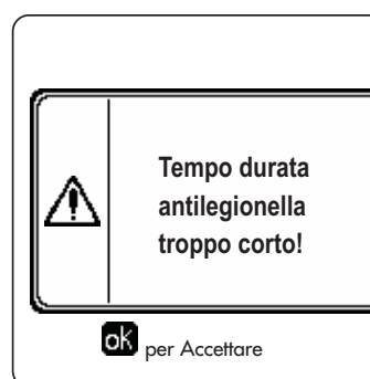
fig. 27- Message Anti-legionella function not completed
