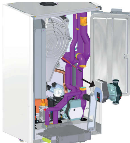
fig. 50 - Replacement/maintenance of the heat pump circulator
